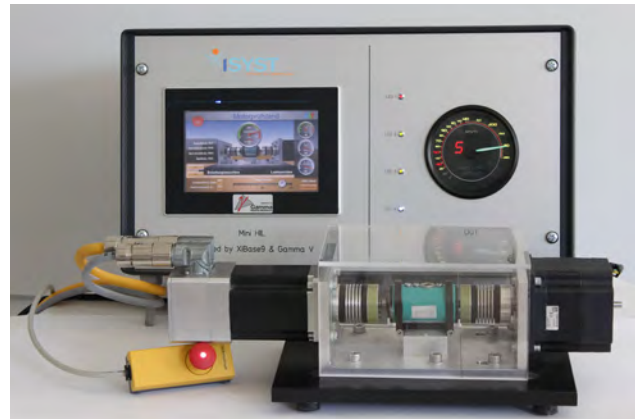
Figure 6: Working environment of an engine test rig (Photo: iSyst)
