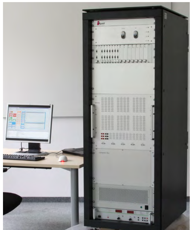
Figure 7: Fullsize HIL system (Photo: iSyst)
