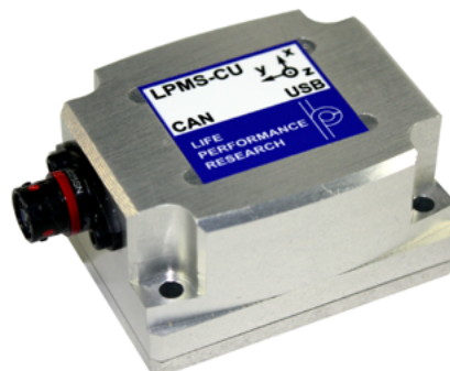
Figure 2: The LPMS-CU is an inertial measurement unit and attitude heading reference system comprising three different 3-axis MEMS (gyroscope, accelerometer, and magnetometer), which provides CAN connectivity (Photo: Life Performance Research)
