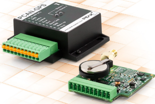
Figure 3: The PCAN-GPS is a CAN-connectable sensor module based on NXP's LPC4000 micro-controller comprising a GPS receiver, a magnetometer, an accelerometer, and a gyroscope (Photo: Peak-System Technik)
